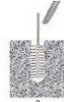
Clean Hole By Brushing And Blowing To Remove All Dust And Debris
